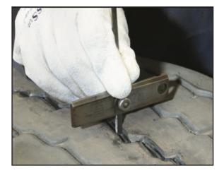
Adjust the depth of cut as specified in this manual. Ensure the width of the blade is set correctly depending upon the tread pattern being cut.
