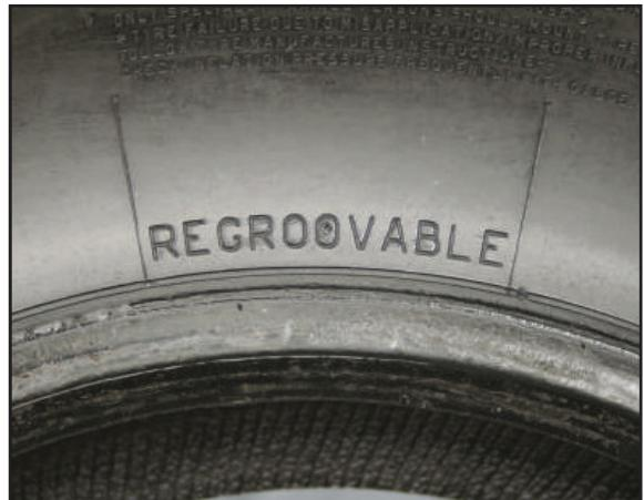
Measure the remaining tread depth at four points around the tyre to determine the minimum amount of remaining tread - there should always be 3-4mm left before regrooving.
